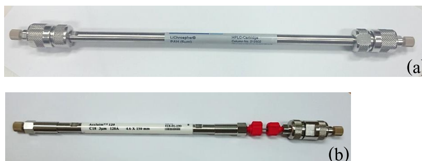
Figure 15 Two Column Types for Chromatographic Separation of Polycyclic Aromatic Hydrocarbons were LiChrospher PAH (a) and Acclaim C18 (b)
